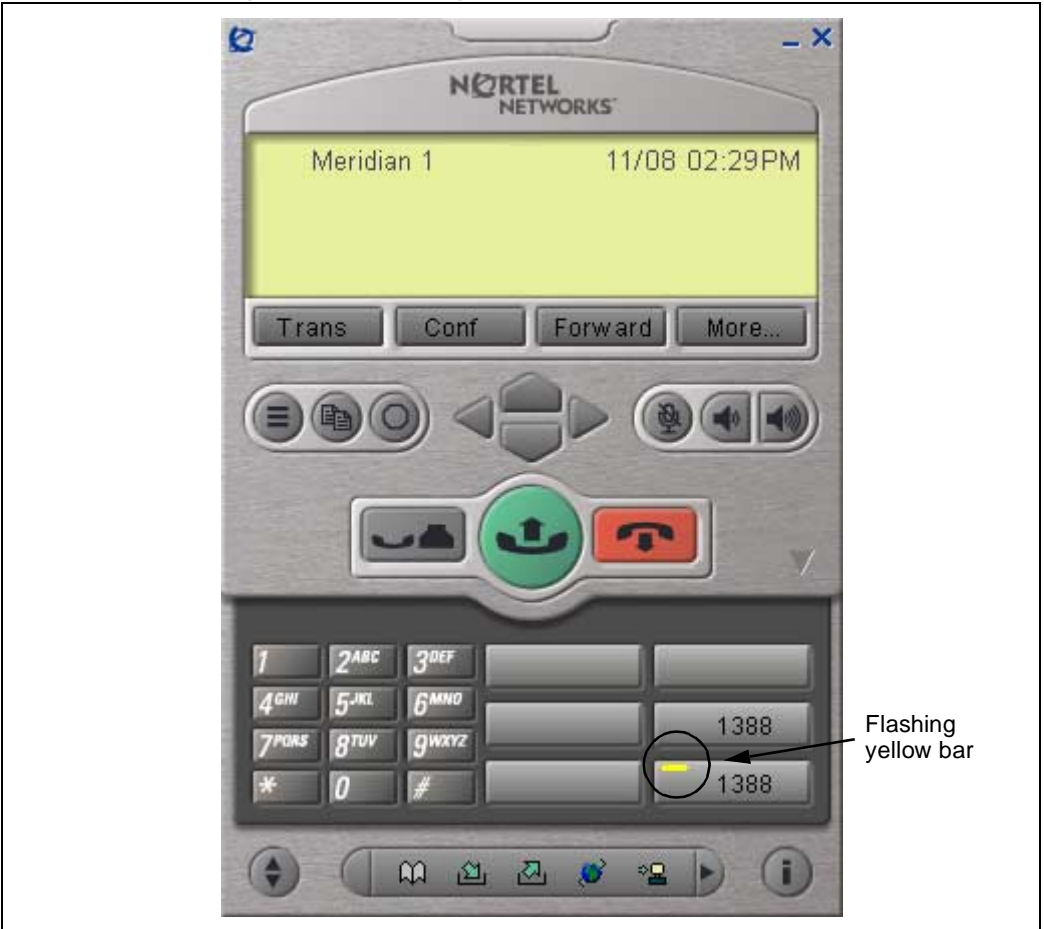
Figure 20 Feature Key indicating hold with flashing yellow bar
